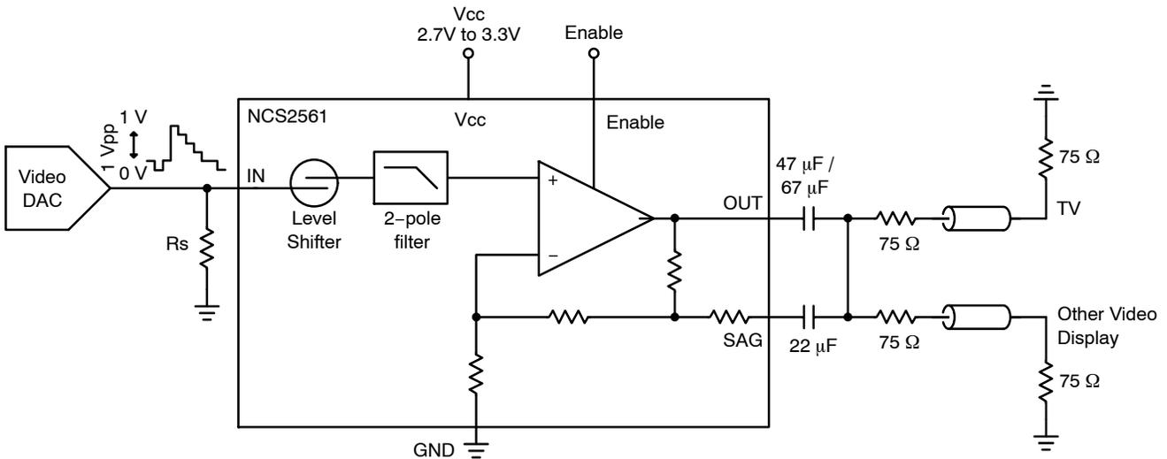
Figure 17. NCS2561 Driving 2 Video Display (two 150 Ω loads)
