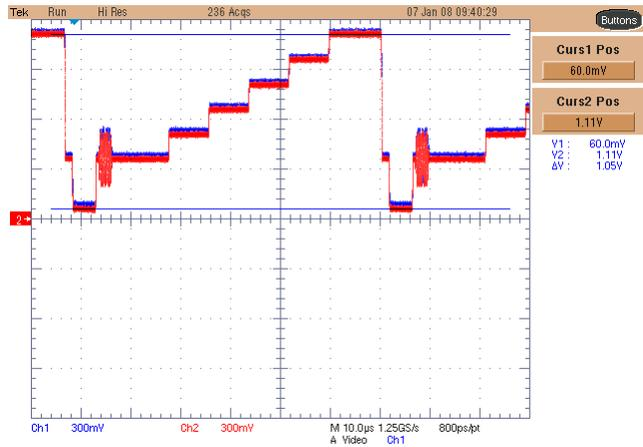
Figure 19. Linearity Test with two 150 Ω loads
