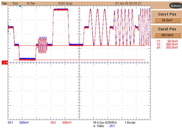
Figure 18. Multiburst Test with two 150 Ω loads
