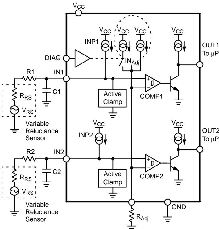
Figure 1. Block Diagram
