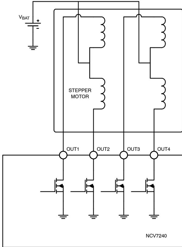
**Figure 34. Stepper Motor Operation Setup**
