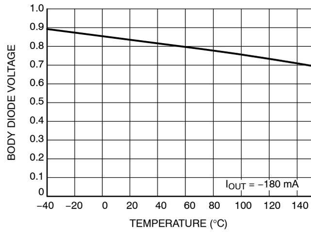
**Figure 18. Output Body Diode Voltage vs. Temperature**
