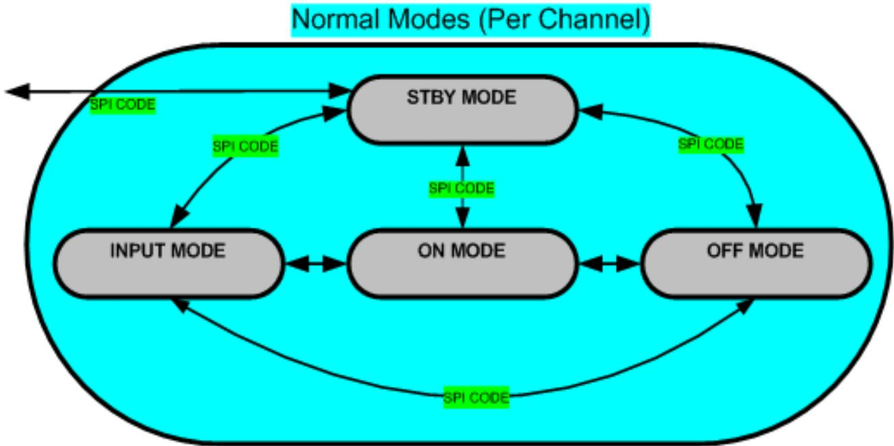
Figure 20. Normal Operation State Diagram
