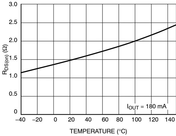
Figure 12. Output  $R_{DS(on)}$  vs. Temperature
