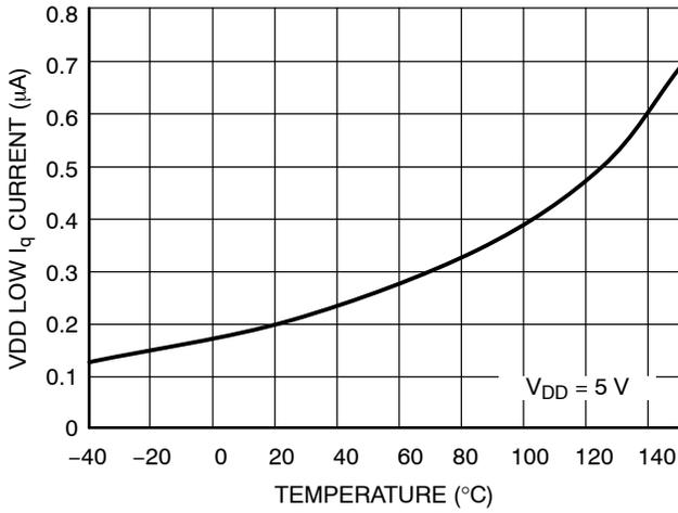
Figure 6. VDD Low I<sub>q</sub> Current vs. Temperature
