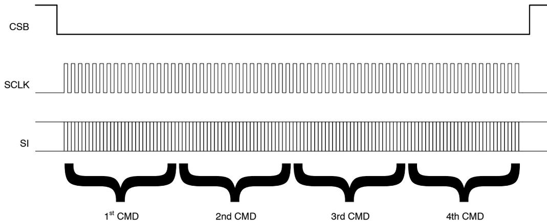
Figure 30. Serial Daisy Chain Timing Diagram
