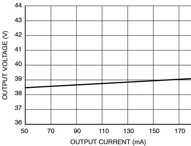
Figure 10. Output Clamp Voltage vs. Current
