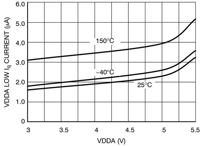
Figure 7. VDDA Low I<sub>q</sub> Quiescent Current vs. VDDA
