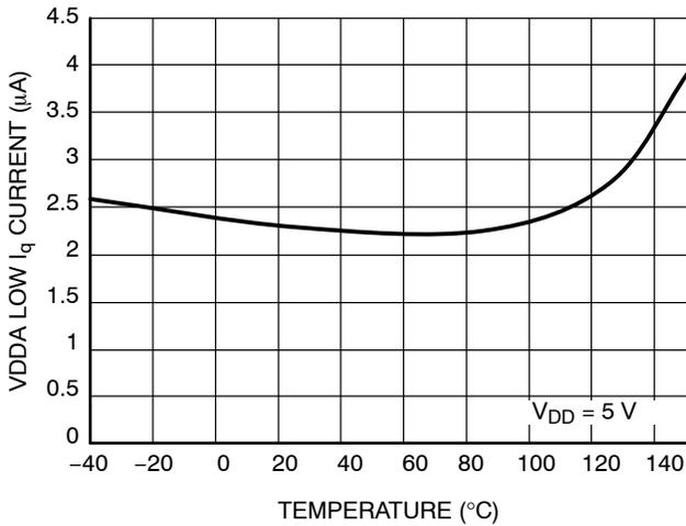
Figure 8. VDDA Low I<sub>q</sub> Current vs. Temperature
