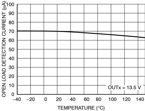
Figure 16. Output Load Detection Current vs. Temperature
