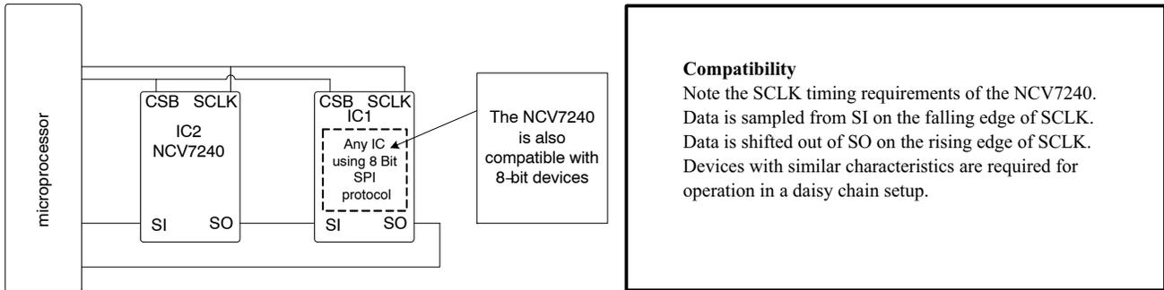
**Figure 31. Serial Daisy Chain with 8-bit Devices**
