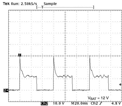
**Figure 35. Typical Stepper Motor Waveform (Unipolar Portescap 35L048L32U)**
