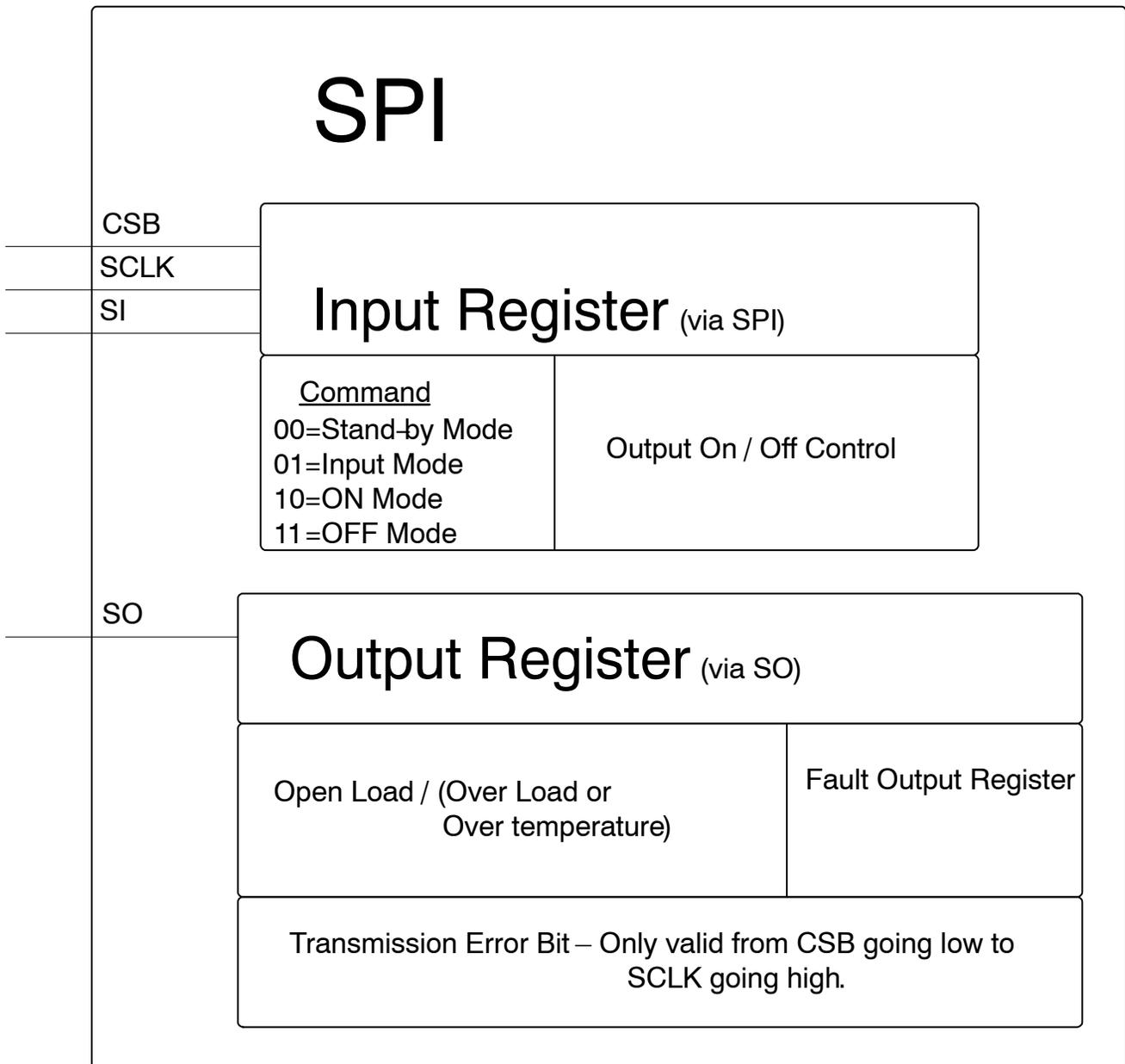
**Figure 36. SPI Register Overview**
