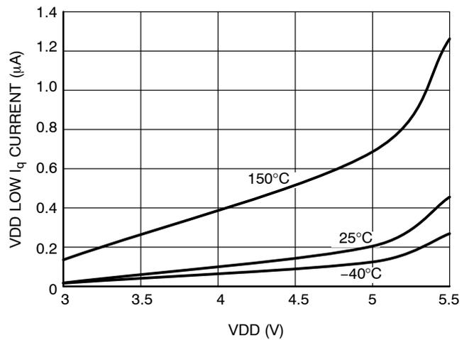
Figure 9. VDD Low I<sub>q</sub> Current vs. VDD
