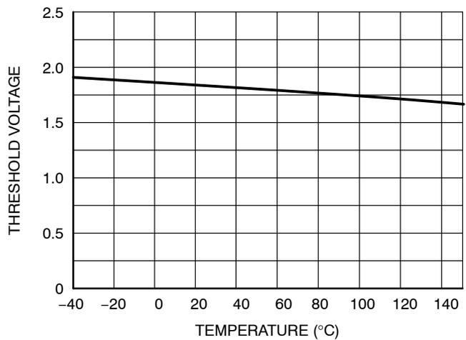
Figure 17. Open Load Detection Voltage vs. Temperature
