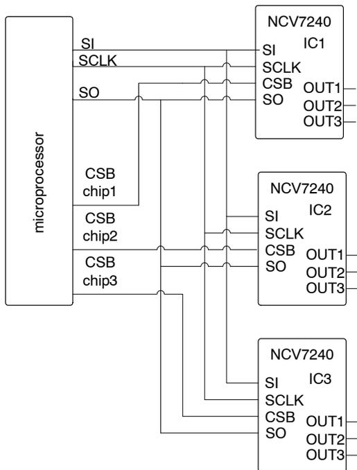
**Figure 32. Parallel Connection**
