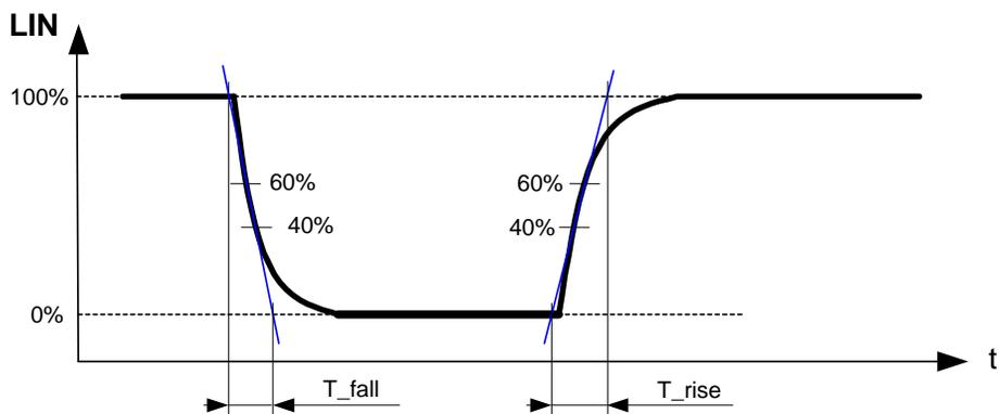
Figure 8. LIN Transmitter Rising and Falling Times
