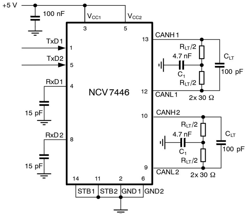
Figure 6. Test Circuit for Timing Characteristics
