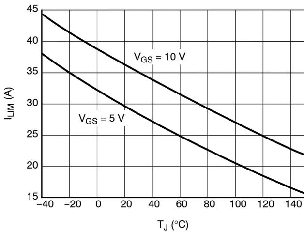
Figure 12. Current Limit vs. Junction Temperature ( $V_{DS} = 10 V$ )
