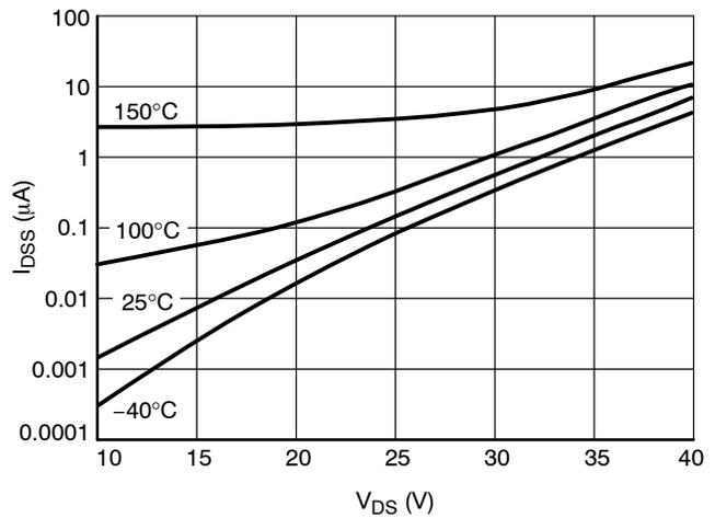
Figure 13. Drain-to-Source Leakage Current ( $V_{GS} = 0 V$ )
