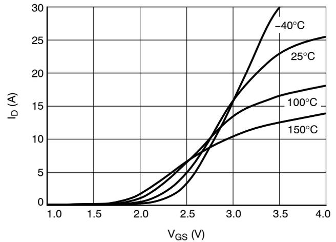
Figure 7. Transfer Characteristics ( $V_{DS} = 10\text{ V}$ )
