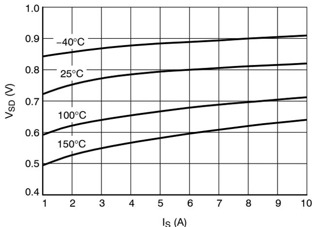
Figure 15. Source-Drain Diode Forward Characteristics ( $V_{GS} = 0 \text{ V}$ )
