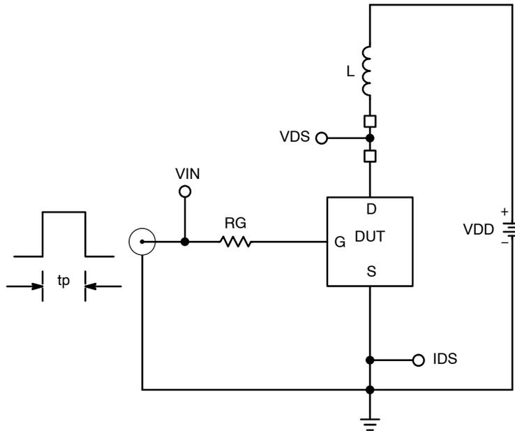
Figure 24. Inductive Load Switching Test Circuit
