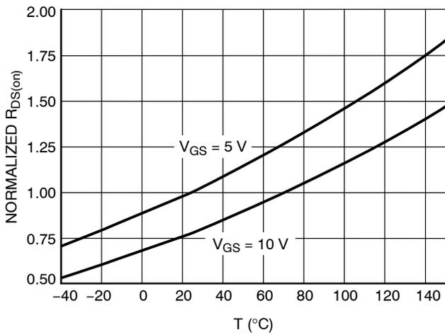
Figure 10. Normalized  $R_{DS(on)}$  vs. Temperature ( $I_D = 5 A$ )
