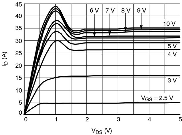
Figure 6. On-state Output Characteristics at 25°C
