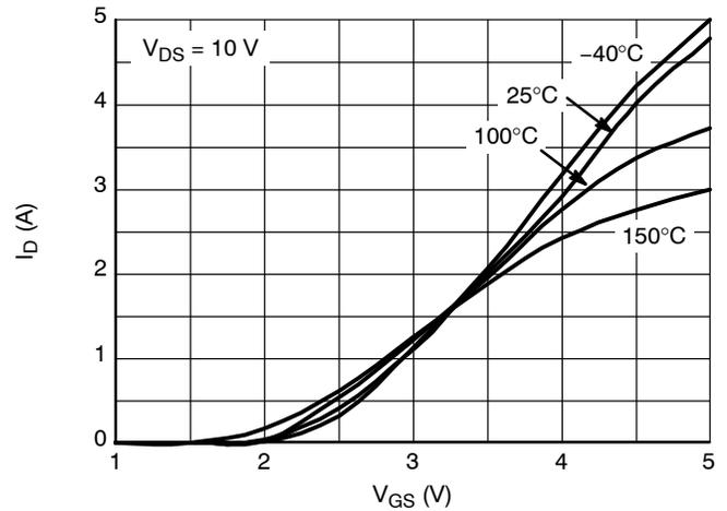
**Figure 7. Transfer Characteristics**
