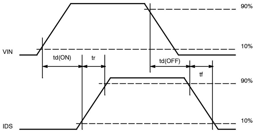
Figure 22. Resistive Load Switching Waveforms
