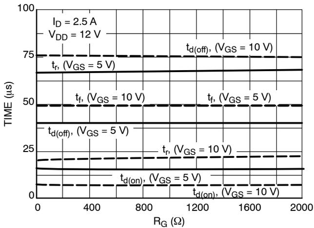
Figure 18. Resistive Load Switching Time vs. Gate Resistance
