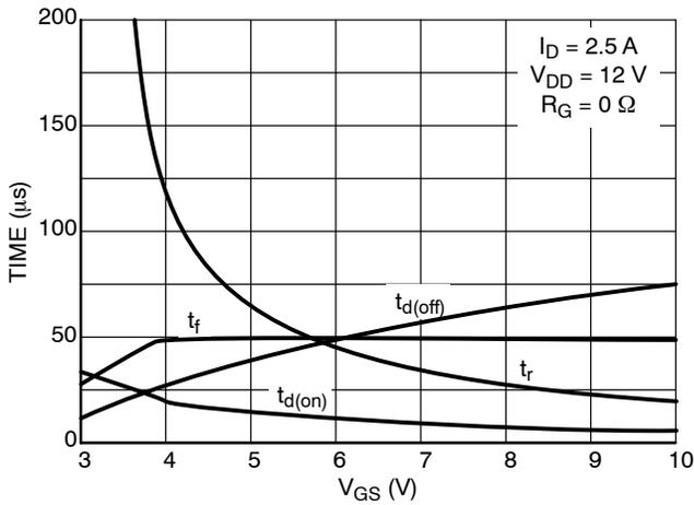
Figure 16. Resistive Load Switching Time vs. Gate-Source Voltage
