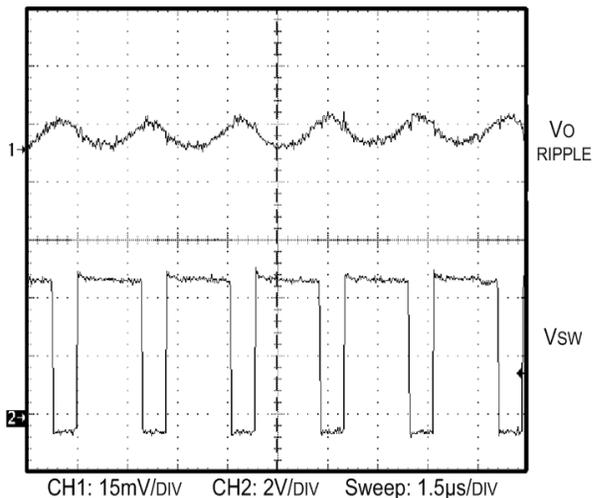
**Figure 15. Output Voltage Ripple Using Two 10 µF Ceramic Capacitors in Parallel**
