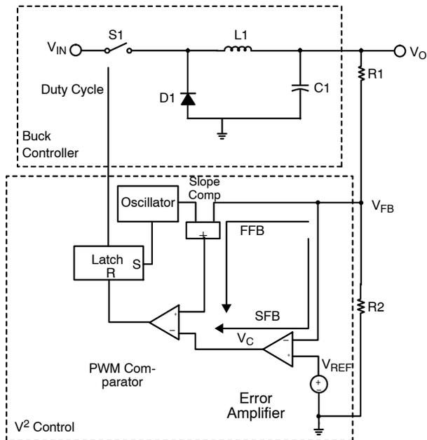
Figure 3. Buck Converter with V<sup>2</sup> Control.
