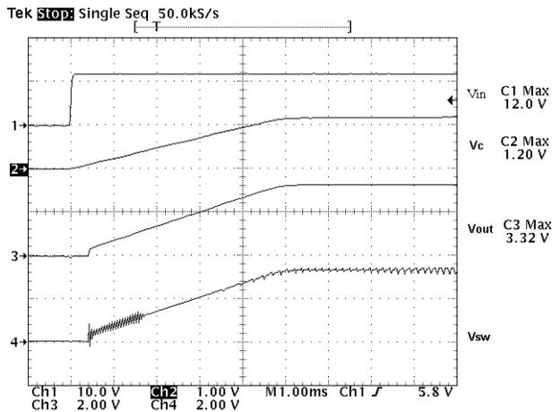
**Figure 11. The Power Up Transition of NCV8843 Regulator**
