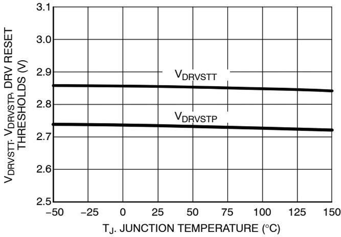
Figure 22. DRV Reset Threshold vs. Junction Temperature
