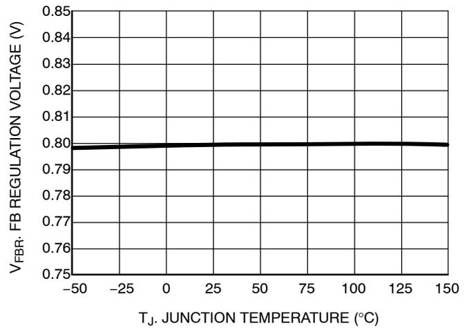
Figure 9. FB Regulation Voltage vs. Junction Temperature
