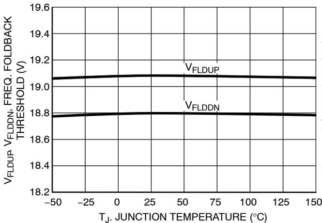
Figure 14. Rising Frequency Foldback Threshold vs. Junction Temperature
