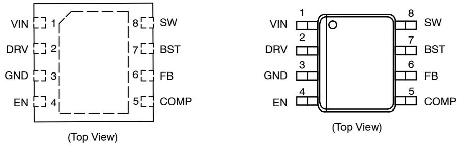
**Figure 3. Pin Connections**
