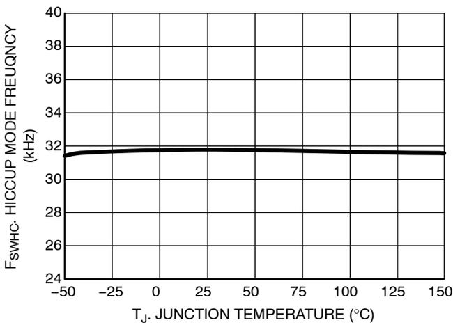
Figure 20. Hiccup Mode Switching Frequency vs. Junction Temperature
