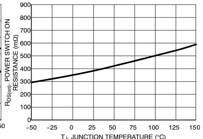
Figure 15. Power Switch  $R_{DS(on)}$  vs. Junction Temperature
