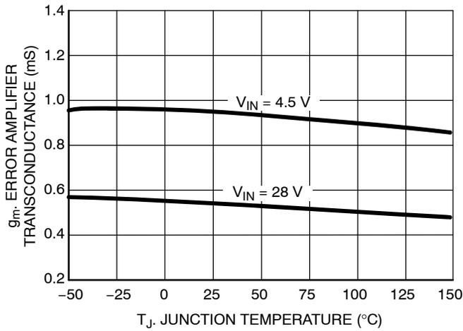
Figure 10. Error Amplifier Transconductance vs. Junction Temperature
