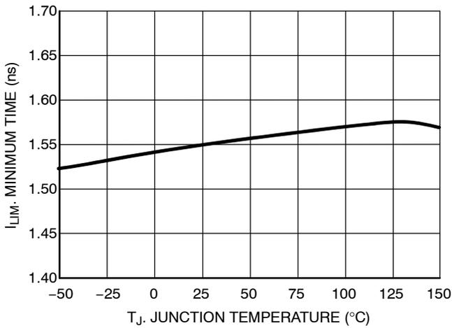
Figure 18. Current Limit Threshold vs. Junction Temperature
