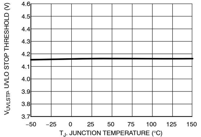
Figure 7. UVLO Stop Threshold vs. Junction Temperature
