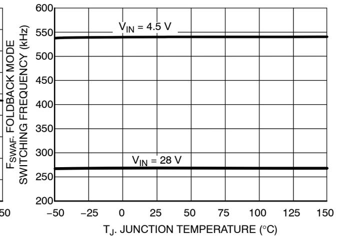
Figure 21. Short-Circuit Foldback Frequency vs. Junction Temperature
