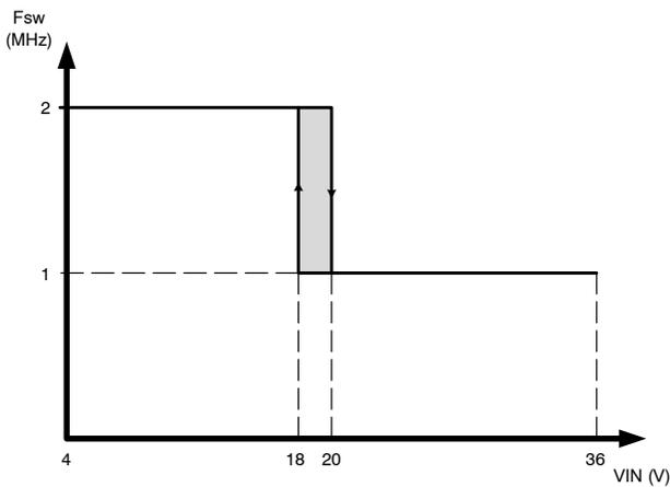
Figure 27. NCV890201 Switching Frequency Reduction at High Input Voltage
