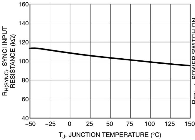
Figure 16. SYNC Input Resistance vs. Junction Temperature
