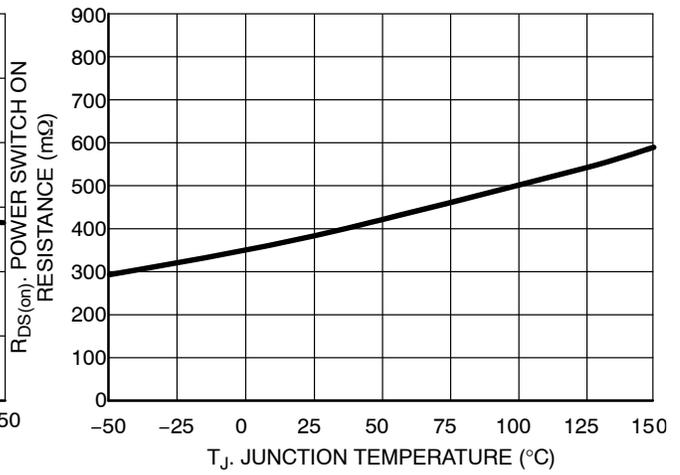
Figure 17. Power Switch R<sub>DS(on)</sub> vs. Junction Temperature
