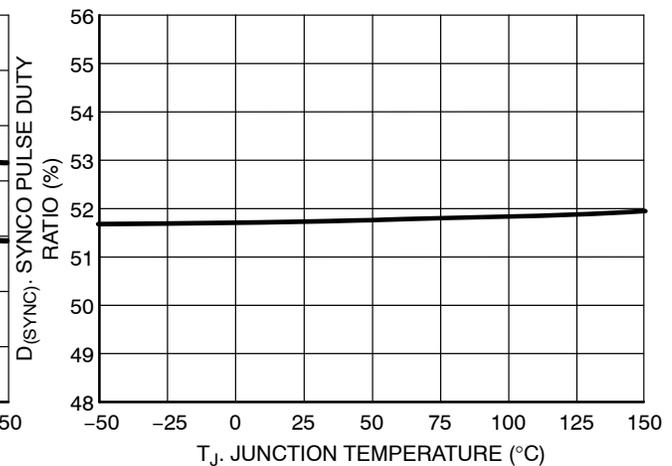
Figure 15. SYNCO Pulse Duty Ratio vs. Junction Temperature
