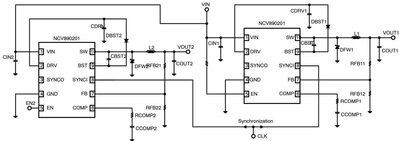
**Figure 30. Both NCV890201s Synchronized to External Clock
