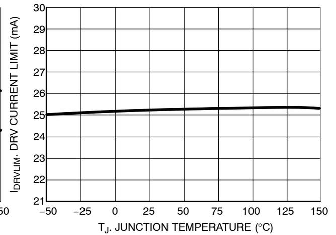
Figure 25. DRV Current Limit vs. Junction Temperature
