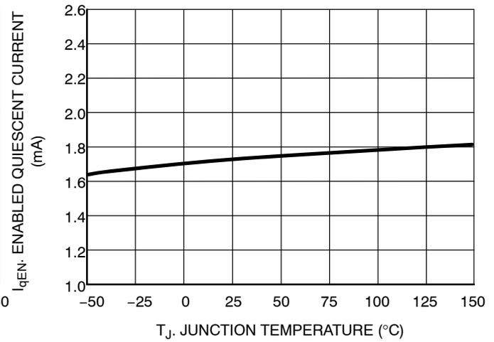
Figure 5. Enabled Quiescent Current vs. Junction Temperature
