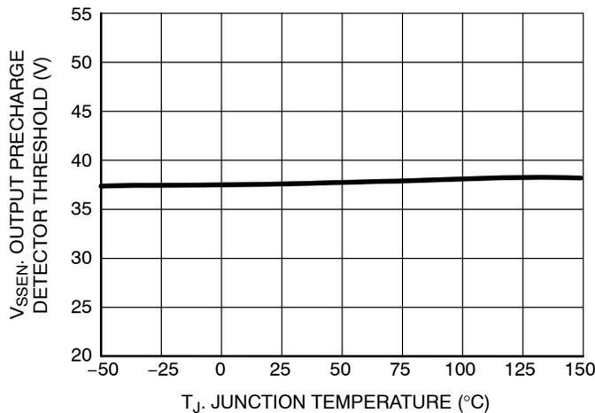
Figure 26. Output Precharge Detector Threshold vs. Junction Temperature
