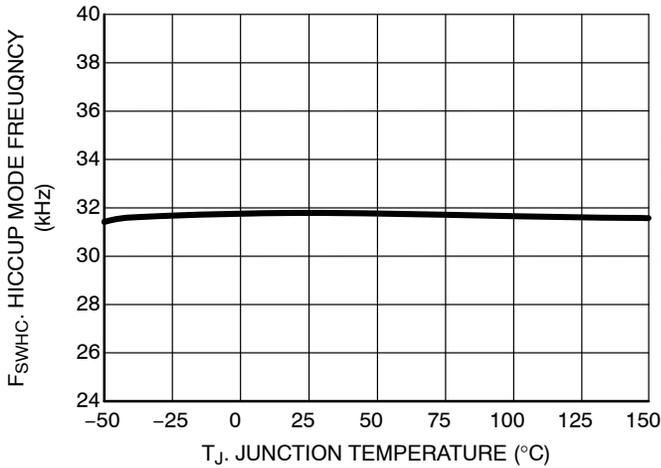
Figure 22. Hiccup Mode Switching Frequency vs. Junction Temperature
