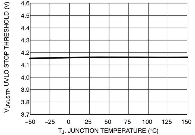
Figure 7. UVLO Stop Threshold vs. Junction Temperature
