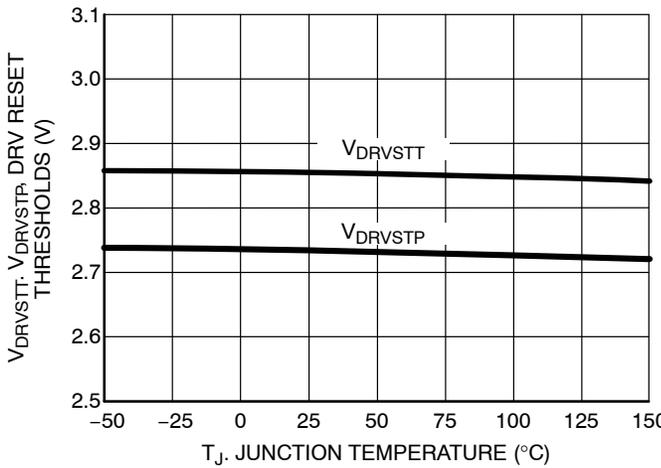
Figure 24. DRV Reset Threshold vs. Junction Temperature
