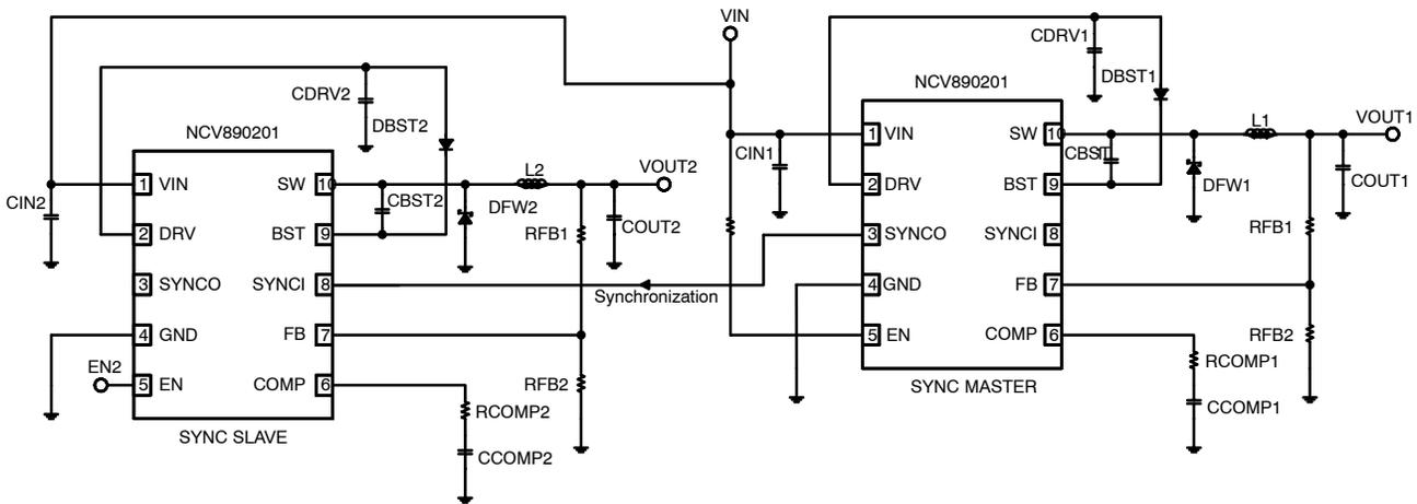
**Figure 29. NCV890201s Synchronized to Each Other
