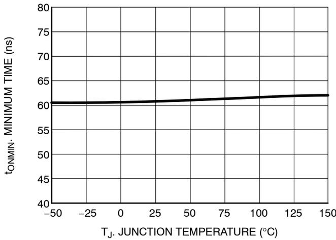
Figure 18. Minimum On Time vs. Junction Temperature
