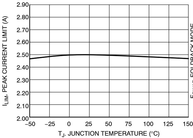
Figure 20. Current Limit Threshold vs. Junction Temperature
