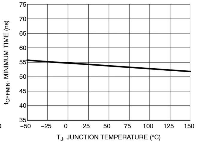
Figure 19. Minimum Off Time vs. Junction Temperature
