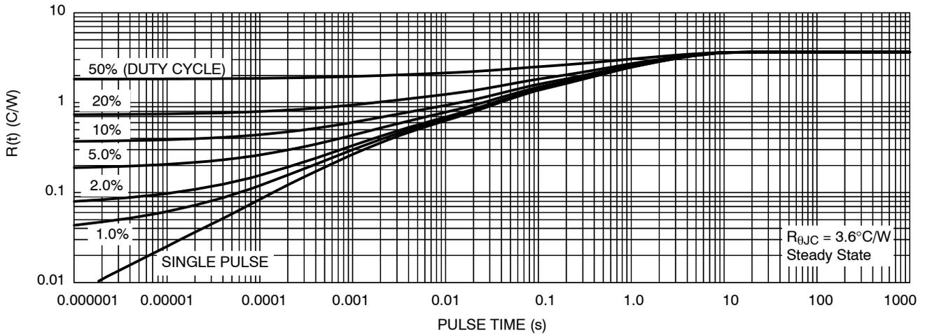
**Figure 13. Thermal Impedance (Junction-to-Case) for NDF08N50Z**
