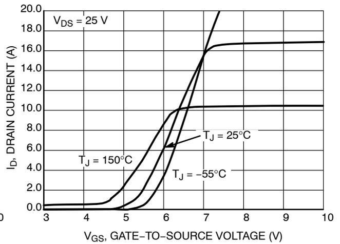
Figure 2. Transfer Characteristics
