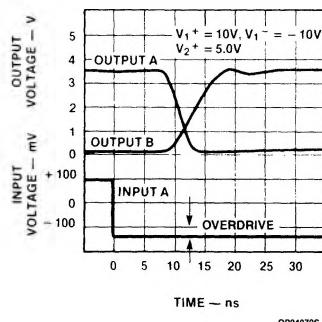
**Response Time For Various Input Overdrives**
