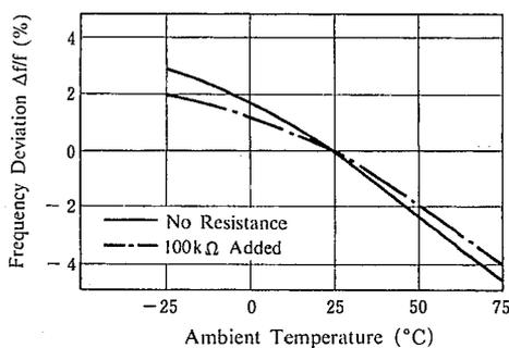
Connection Resistance between pin 1 and 12
