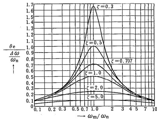
Fig. 4 Steady-state Phase Error by Sine Wave FM
