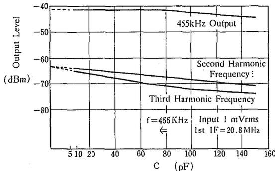
**Graph-8 Change of Input Sensitivity by Pin (6) Decoupling Capacitor**
