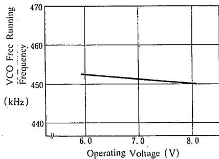
**Graph 16 VCO Free Running Frequency Deviation vs. Operating Voltage**
