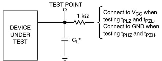
\*Includes all probe and jig capacitance.
