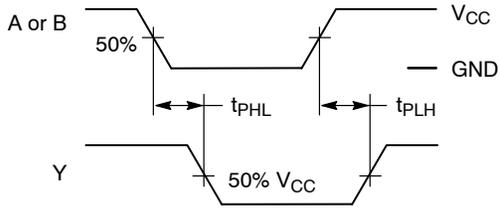
**Figure 3. Switching Waveform**
