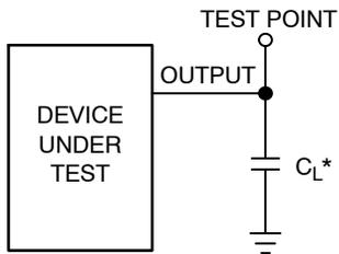
\*Includes all probe and jig capacitance.
