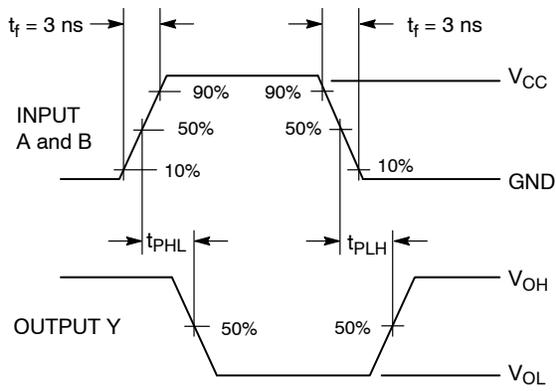
**Figure 3. Switching Waveform**
