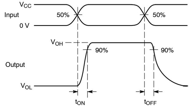
Figure 5.  $t_{ON}/t_{OFF}$
