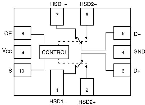
**Figure 1. Pin Connections and Logic Diagram**
