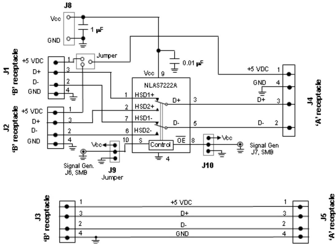
Figure 8. Schematic of the NLAS7222B USB Demo Board
