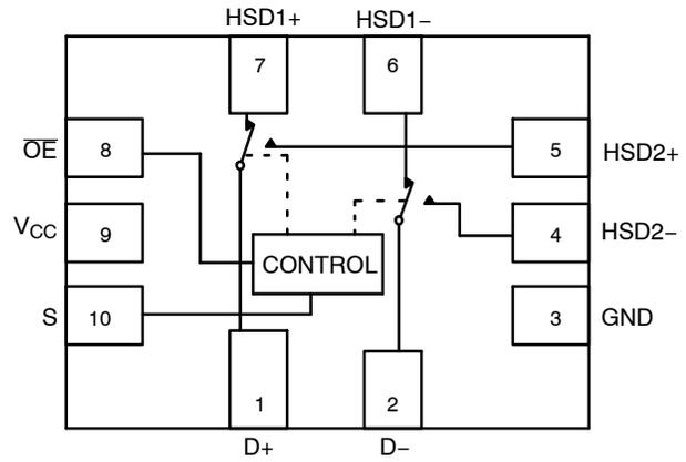
**Figure 2. Pin Connections and Logic Diagram**
