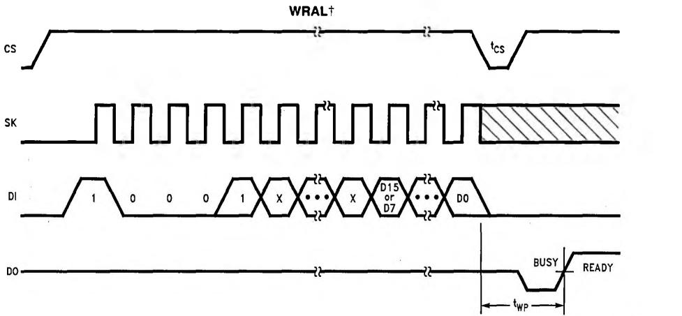
†For the EWEN, EWDS, WRAL and ERAL it is necessary to provide a minimum number of clock cycles after the last bit of opcode is clocked in. In the 64x16 configuration a minimum of 4 additional clock cycles are required. In the 128 x 8 configuration a minimum of 5 additional clock cycles are required.
