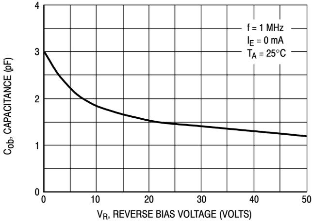
Figure 9. Output Capacitance
