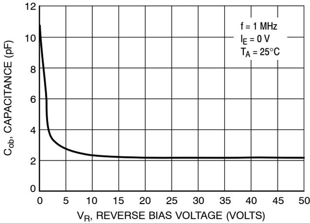
Figure 4. Output Capacitance
