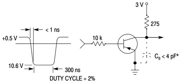
**Figure 1. Delay and Rise Time Equivalent Test Circuit**
