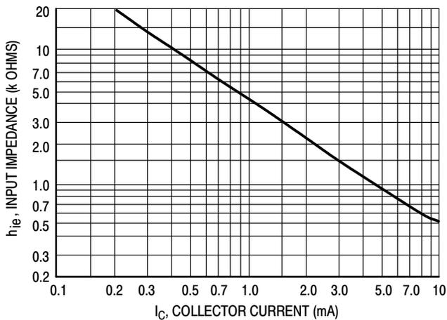
Figure 10. Input Impedance
