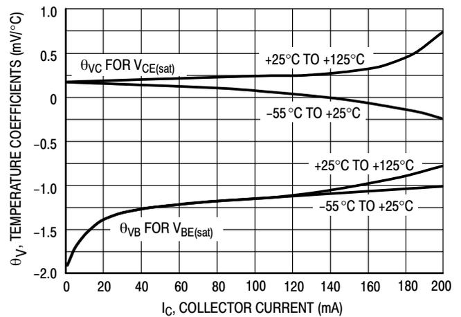
Figure 15. Temperature Coefficients
