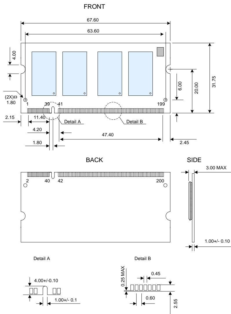
Note: All dimensions are typical with tolerances of +/- 0.15 unless otherwise stated.
