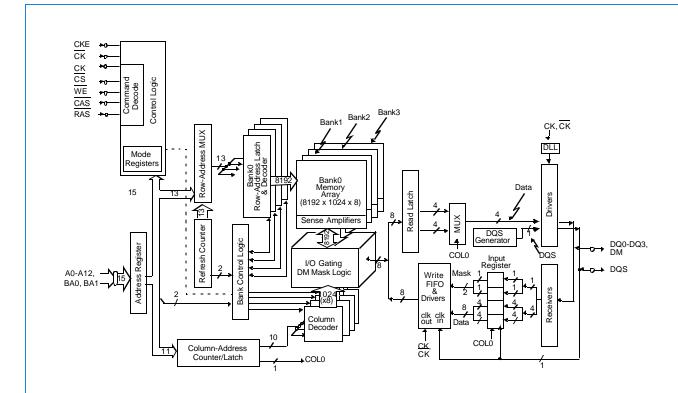
**Note:** This Functional Block Diagram is intended to facilitate user understanding of the operation of the device; it does not represent an actual circuit implementation.
