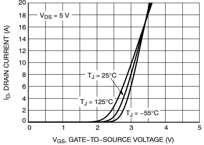
Figure 2. Transfer Characteristics
