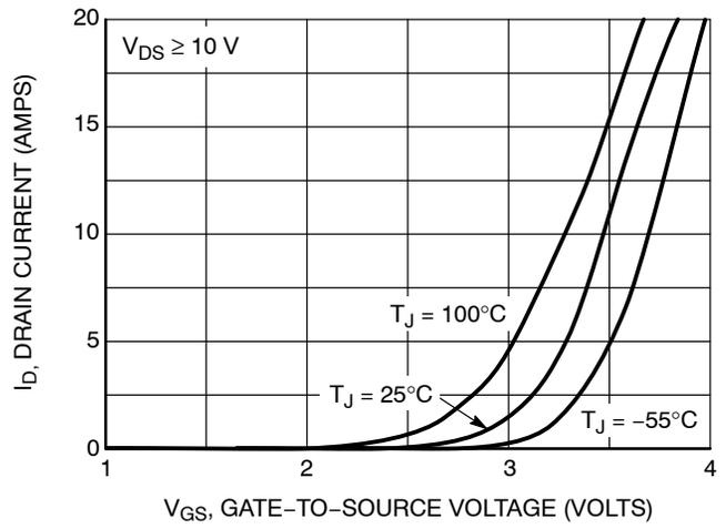
Figure 2. Transfer Characteristics
