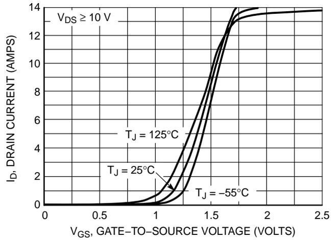
**Figure 2. Transfer Characteristics**
