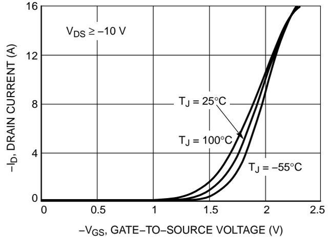
Figure 2. Transfer Characteristics
