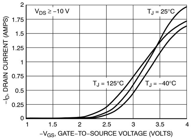
Figure 2. Transfer Characteristics
