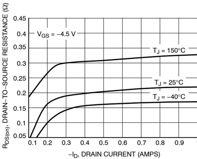
Figure 3. On-Resistance versus Drain Current and Temperature
