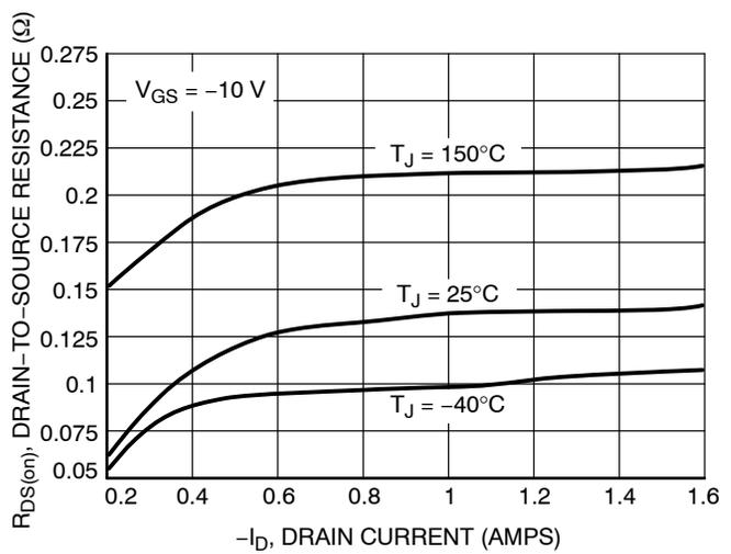
Figure 4. On-Resistance versus Drain Current and Temperature
