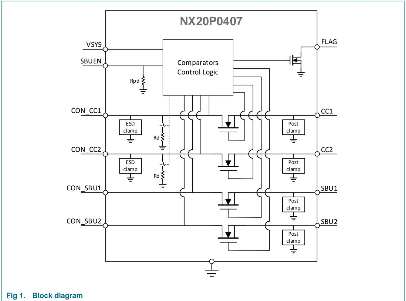
**Fig 1. Block diagram**
