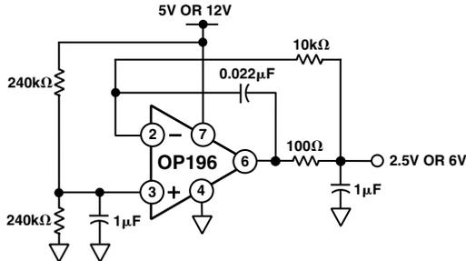
Figure 5. A Micropower False-Ground Generator
