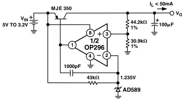
Figure 8. 3 V Low Dropout Voltage Regulator
