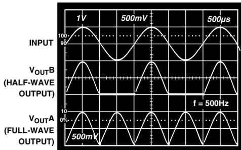
Figure 6. Single-Supply Half-Wave and Full-Wave Rectifiers Using an OP296
