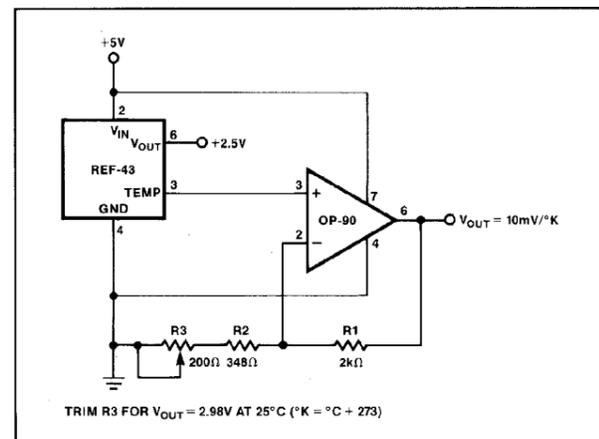
FIGURE 9: Thermocouple Amplifier with Cold-Junction Compensation
