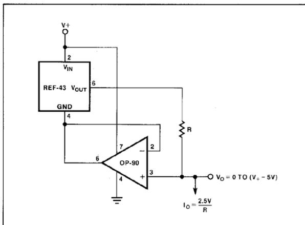
FIGURE 8: Single-Supply Kelvin-Output Thermometer
