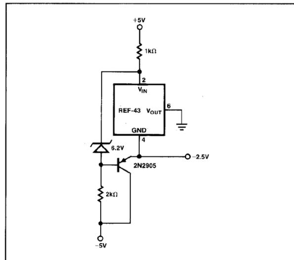
element is a PNP transistor, with the REF-43 in a servo loop to ensure that the output remains 2.5V below ground.
