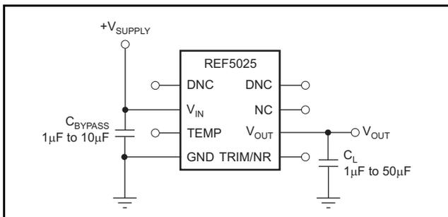
Figure 25. Basic Connections
