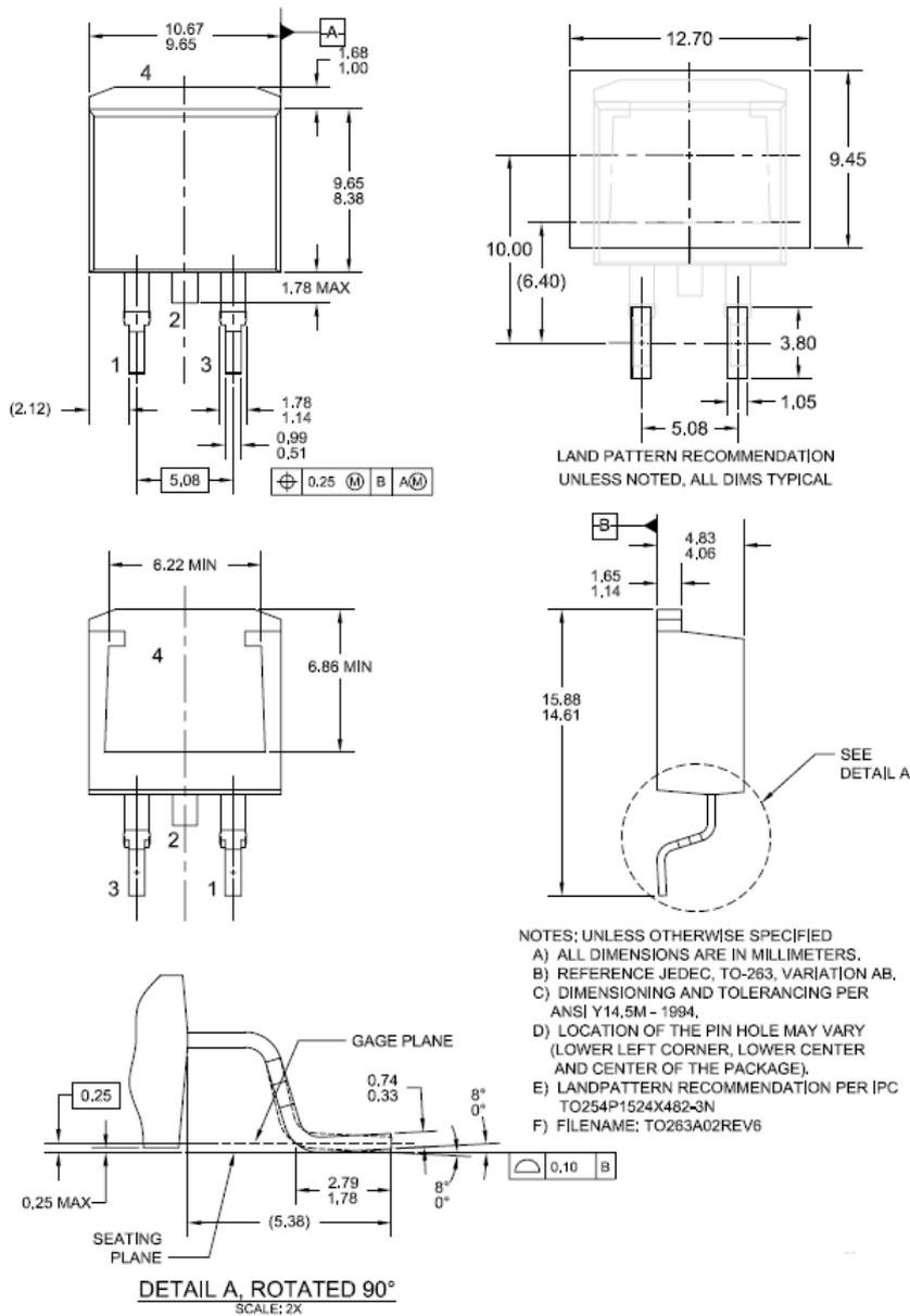
Figure 19. TO-263 2L (D2PAK) - 2LD, TO263, SURFACE MOUNT
