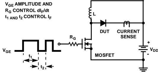
Figure 12.  $t_{rr}$  Test Circuit
