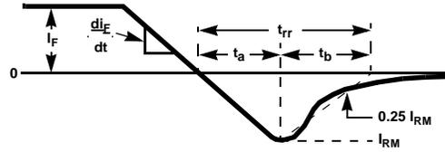
Figure 13.  $t_{rr}$  Waveforms and Definitions
