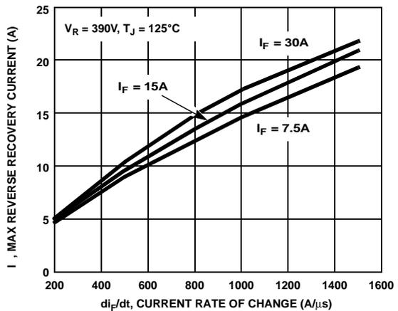
Figure 6. Maximum Reverse Recovery Current vs  $di_F/dt$
