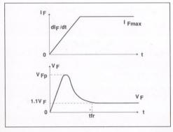
Turn-on losses : (in the transistor, due to the diode)
