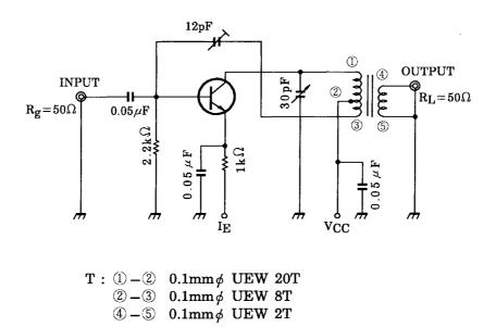
Figure 1 NF, Gpe Test Circuit
