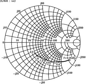
$\begin{array}{l} S_{11e} \\ V_{CE} = 10V \\ I_{C} = 20 mA \\ T_{a} = 25^{\circ}C \\ (Unit: \Omega) \end{array}$
