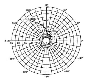
$\begin{array}{l} S_{12e} \\ V_{CE} = 10V \\ I_{C} = 20 mA \\ Ta = 25 ^{\circ}C \end{array}$
