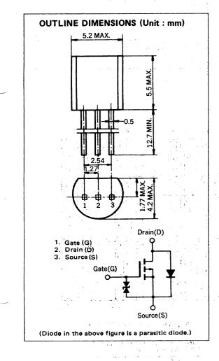
The 2SJ198 is a p-channel vertical type MOS FET switching device which can be directly driven from an IC operating with a 5 V single power supply. The device featuring low ON-state resistance is of the voltage drive type and thus is ideal for driving actuators such as motors, solenoids, and relays.
