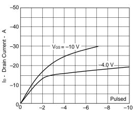
V<sub>DS</sub> - Drain to Source Voltage - V
