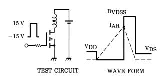
$$\begin{array}{l} Peak~I_{AR} = 3~A,~R_G = 25~\Omega \\ V_{DD} = 90~V,~L = 60~mH \end{array} \quad E_{AS} = \frac{1}{2} \cdot L \cdot I^2 \cdot (~\frac{BVDSS}{BVDSS - V_{DD}}) \label{eq:peak}$$
