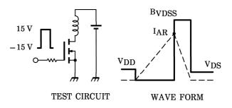
$$\begin{array}{l} \text{Peak I}_{AR} = 18 \text{ A, } R_G = 25 \, \Omega \\ \text{V}_{DD} = 50 \, \text{V, L} = 0.8 \, \text{mH} \end{array} \quad \text{E}_{AS} = \frac{1}{2} \cdot \text{L} \, \cdot \text{I}^2 \cdot (\, \frac{\text{BVDSS}}{\text{BVDSS} - \text{VDD}}) \end{array}$$
