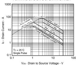
DRAIN CURRENT vs. DRAIN TO SOURCE VOLTAGE Pulsed 100 lo - Drain Current - A 80 Vgs=10 V 60 4.5 V 40
