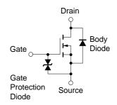
The diode connected between the gate and source of the transistor serves as a protector against ESD.
