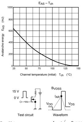
$\begin{array}{ll} R_G = 25 \; \Omega \\ V_{DD} = 50 \; V, \; L = 350 \; \mu H \end{array} \qquad \qquad \\ E_{AS} = \frac{1}{2} \cdot L \cdot l^2 \cdot \left( \frac{B_{VDSS}}{B_{VDSS} - V_{DD}} \right) \end{array}$
