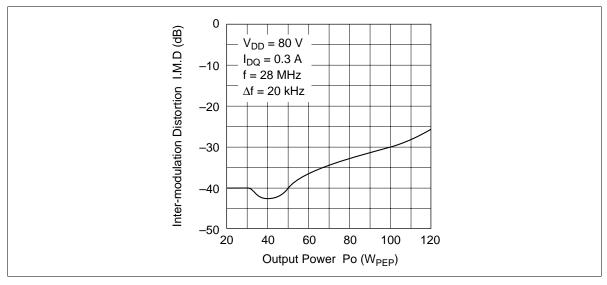
Figure 10 Inter-Modulation Distortion vs. Output Power
