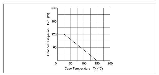
Figure 1 Power vs. Temperature Derating
