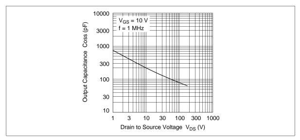
Figure 7 Output Capacitance vs. Drain to Source Voltage
