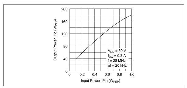
Figure 9 Output Power vs. Input Power (2 Tones)
