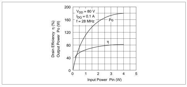
Figure 8 Output Power, Drain Efficiency vs. Input Power
