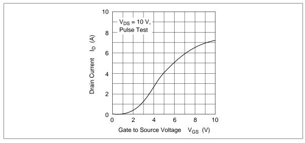
Figure 4 Typical Transfer Characteristics
