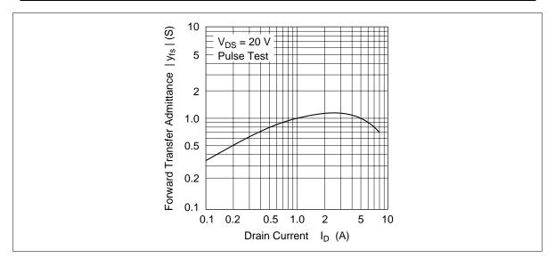
Figure 5 Forward Transfer Admittance vs. Drain Current
