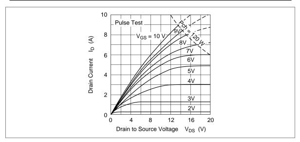
Figure 3 Typical Output Characteristics
