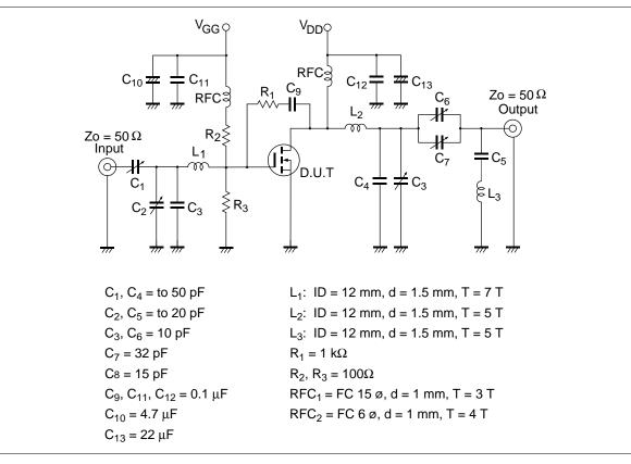
Figure 11 28 MHz Pout Test Circuit
