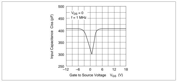
Figure 6 Input Capacitance vs. Gate to Source Voltage
