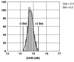
**Figure 4. Gain @ 2 GHz, 4 V, 80 mA.** LSL=13.5, Nominal=14.8, USL=16.5
