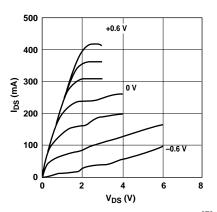
Figure 1. Typical Pulsed I-V Curves<sup>[7]</sup>.  $(V_{GS} = -0.2 V \text{ per step})$
