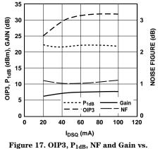
Figure 17. OIP3, P<sub>1dB</sub>, NF and Gain vs. Bias<sup>[1,2]</sup> at 5.8 GHz.
