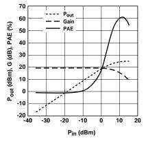
Figure 20. Swept Power Tuned for Max  $P_{1dB}$  $V_{DS}$  = 4V,  $I_{DSQ}$  = 80 mA, 2 GHz.
