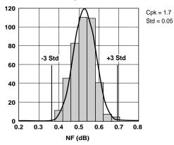
**Figure 2. NF @ 2 GHz, 4 V, 80 mA.** LSL=0.2, Nominal=0.53, USL=0.8
