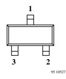
BF569 Marking: LH Plastic case (SOT 23) 1= Collector; 2= Base; 3= Emitter BF569R Marking: LM Plastic case (SOT 23) 1= Collector; 2= Base; 3= Emitter
