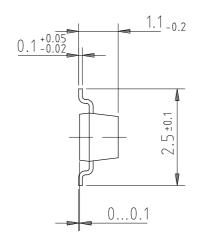
96 12240 technical drawings according to DIN specifications
