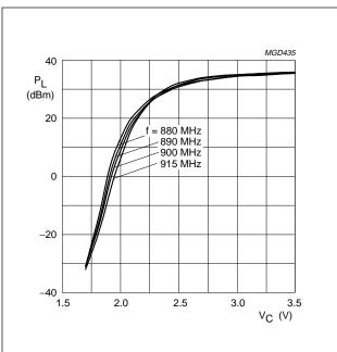
$$\begin{split} & Z_{S} = Z_{L} = 50 \; \Omega; \; P_{D} = 1 \; mW; \; V_{S1} = V_{S2} = 6 \; V; \\ & T_{mb} = 25 \; ^{\circ}C; \; \delta = 1:8; \; t_{p} = 575 \; \mu s. \end{split}$$
