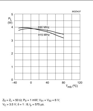
Fig.5 Load power as a function of mounting base temperature; typical values.
