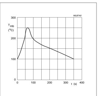
Fig.12 Maximum allowable temperature profile.
