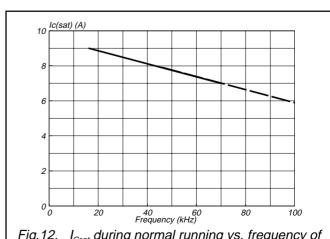
Fig.12. I<sub>Csat</sub> during normal running vs. frequency of operation for optimum performance
