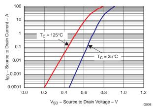
Figure 9. Typical Diode Forward Voltage
