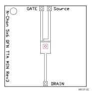
Max  $R_{\theta JA} = 121^{\circ} C/W$  when mounted on minimum pad area of 2-oz. (0.071-mm thick) Cu.
