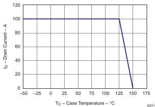
Figure 12. Maximum Drain Current vs. Temperature
