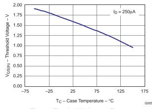
Figure 6. Threshold Voltage vs. Temperature
