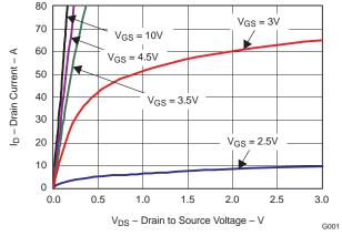
Figure 2. Saturation Characteristics
