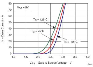
Figure 3. Transfer Characteristics
