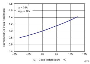
Figure 8. On Resistance vs. Temperature
