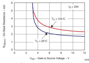
Figure 7. On Resistance vs. Gate Voltage
