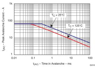
Figure 11. Single Pulse Unclamped Inductive Switching
