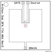
Max  $R_{\theta JA} = 51^{\circ} C/W$  when mounted on 1 inch² (6.45 cm²) of 2-oz. (0.071-mm thick) Cu.
