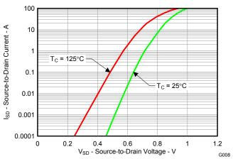
Figure 9. Typical Diode Forward Voltage
