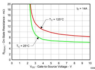
Figure 7. On-State Resistance vs. Gate-to-Source Voltage
