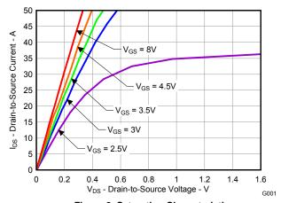
Figure 2. Saturation Characteristics
