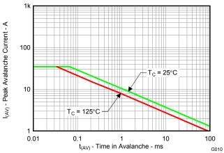
Figure 11. Single Pulse Unclamped Inductive Switching
