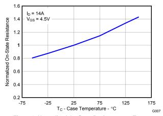
Figure 8. Normalized On-State Resistance vs. Temperature
