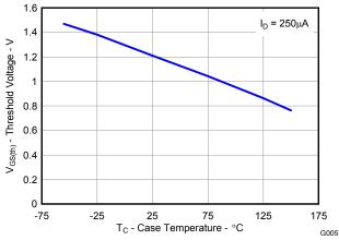
Figure 6. Threshold Voltage vs. Temperature
