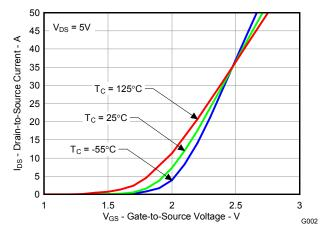
Figure 3. Transfer Characteristics
