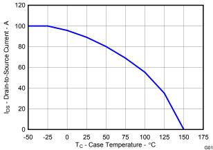
Figure 12. Maximum Drain Current vs. Temperature
