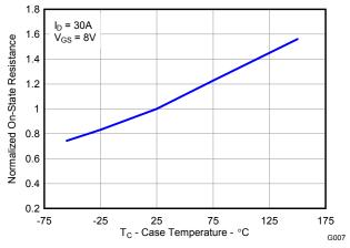
Figure 8. Normalized On-State Resistance vs. Temperature
