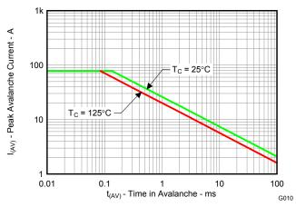
Figure 11. Single Pulse Unclamped Inductive Switching
