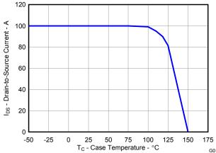
Figure 12. Maximum Drain Current vs. Temperature
