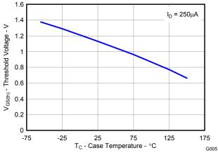
Figure 6. Threshold Voltage vs. Temperature
