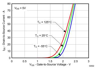
Figure 3. Transfer Characteristics
