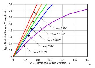
Figure 2. Saturation Characteristics
