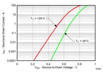
Figure 9. Typical Diode Forward Voltage
